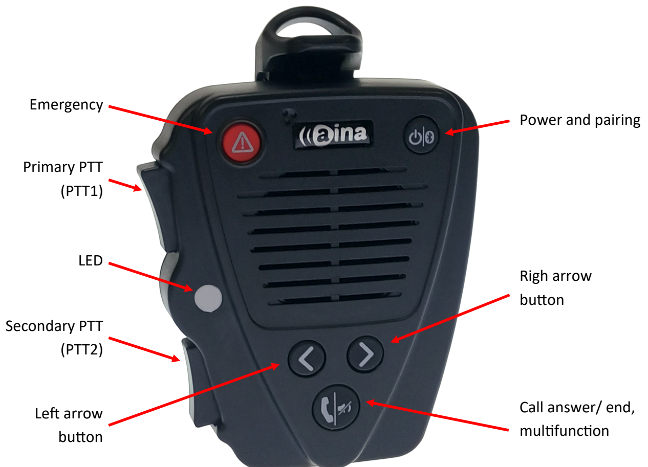
Figure 1: Controls and indicators
