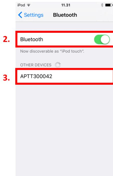
**NOTE:** The Voice Responder can only be paired with one device at a time. If you want to pair it to another device you need to perform an **Unpairing/ Software reset** by pressing and holding both soft buttons and both PTT buttons simultaneously, until the LED blinks once in yellow.
