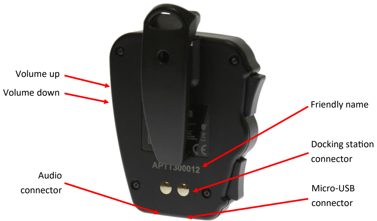
Figure 2: Rear view and connectors
